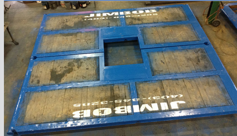
2 - 8' X 20' Mats with 4' X 4' Opening for Wellhead
